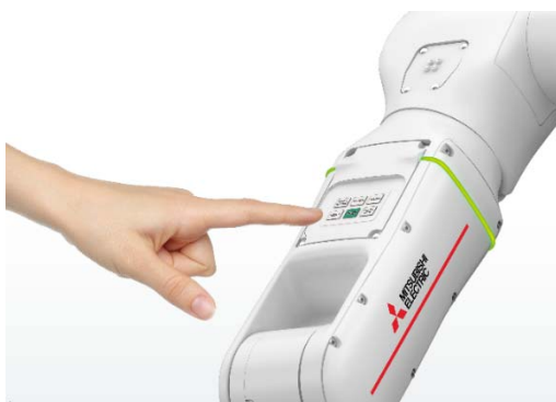
Dedicated control panel on robot arm enables robot movements to be taught and recorded easily
