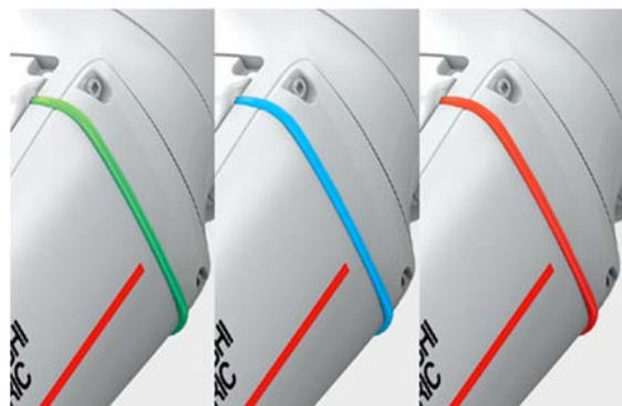
Bright LED light clearly indicates robot status
