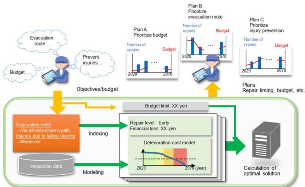
Fig. 1 New technology for preparing maintenance management plans
