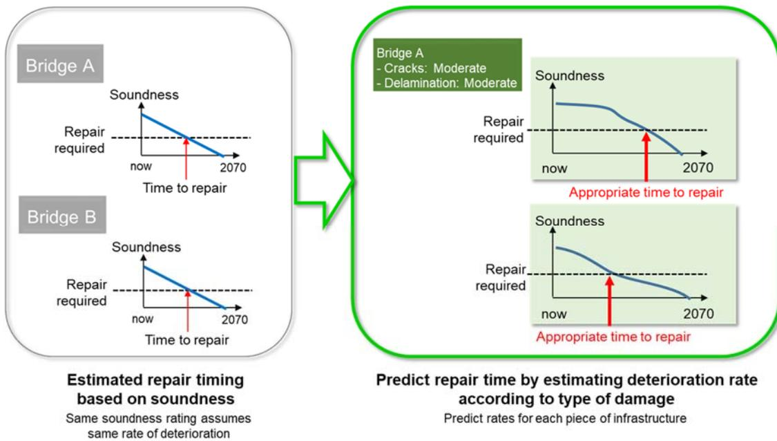
Fig. 2 Prediction repair timing using deterioration-rate model
