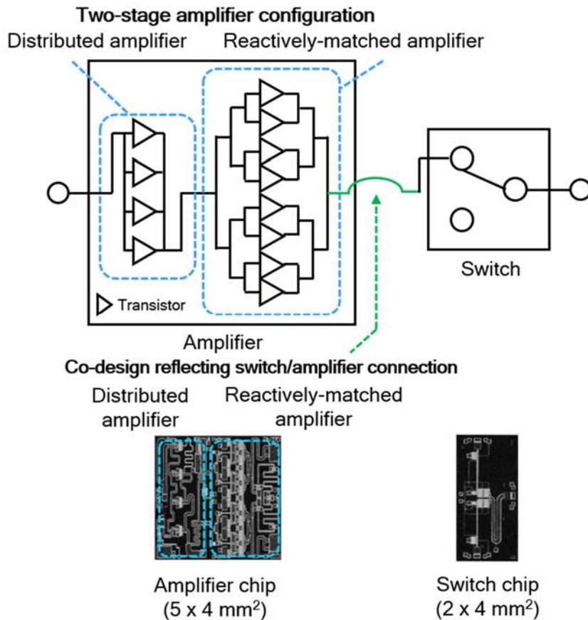
Fig. 2 Ultra-wideband transmission chipset features
