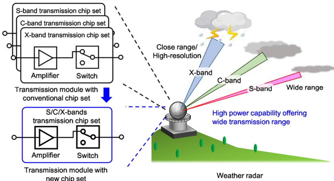
Fig. 1 Multi-purpose wireless system utilizing ultra-wideband chip set
