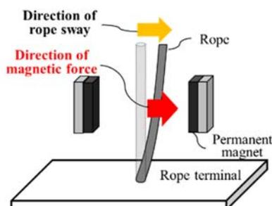
① The permanent magnet applies a magnetic force to the rope near the rope terminal so as to amplify the rope sway.
