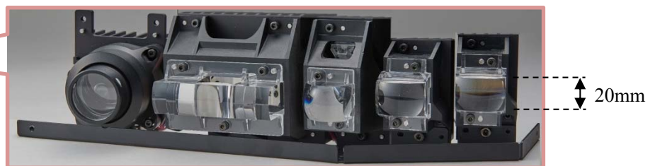
Compact, flexible and highly efficient optical module for LED headlights
