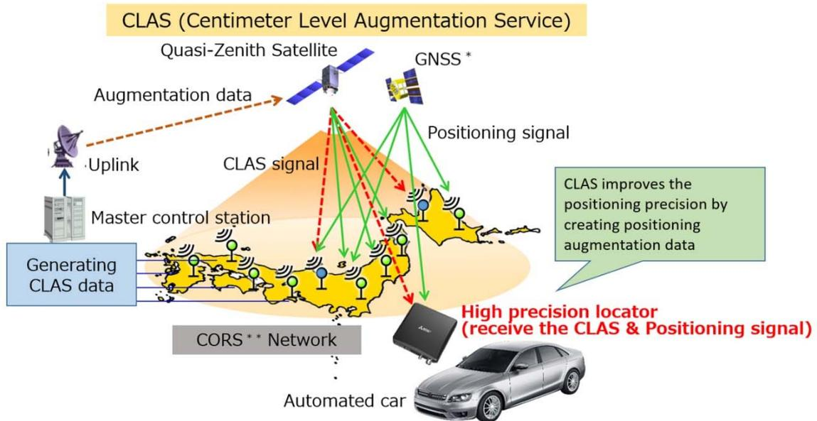
CLAS is a positioning-augmentation service for high-precision positioning, distributed free of charge in Japan from the QZSS, which operates under the auspices of the Cabinet Office. CLAS is scheduled to begin operating in April 2018 and is currently in the final stages of verification. It is expected to be used for practical applications such as safe-driving assistance and automated driving.
