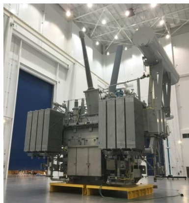
High-capacity 765kV transformer
