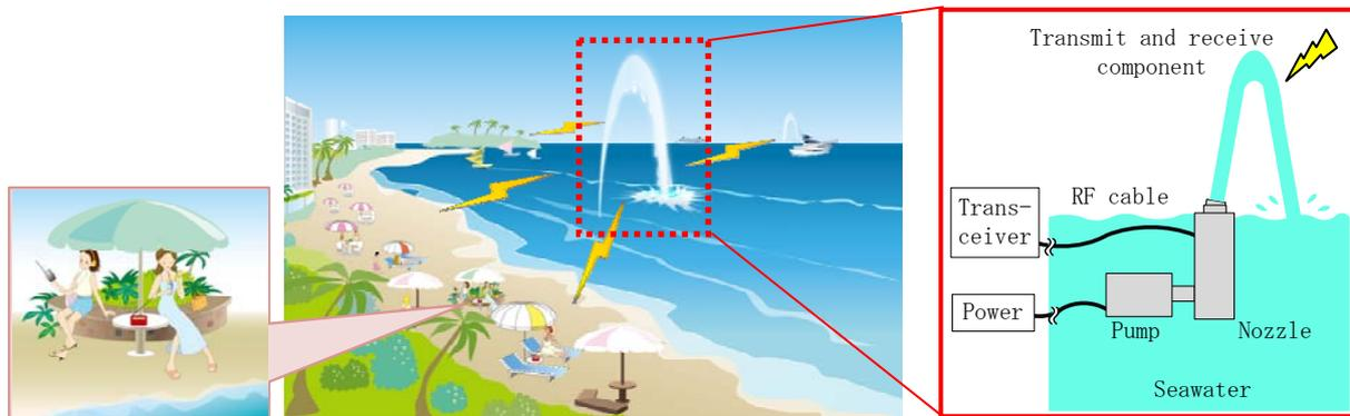
A plume of seawater can be used as an antenna if it is insulated, so Mitsubishi Electric developed an insulated nozzle that transmits radio waves to the antenna even when the plume is physically connected to the sea surface. Effective insulation is achieved with a quarter-wavelength tube in the nozzle.
